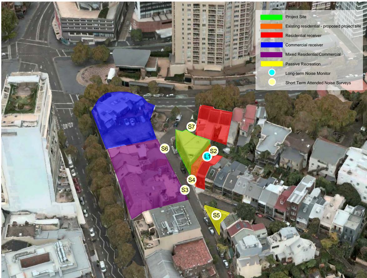
Figure 6: The Project site in relation to noise-sensitive receivers, and locations for both unattended long-term noise monitoring and attended short-term noise measurements
